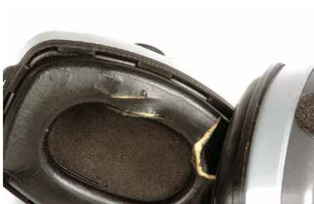
Figure 36 Damaged earmuff seal
