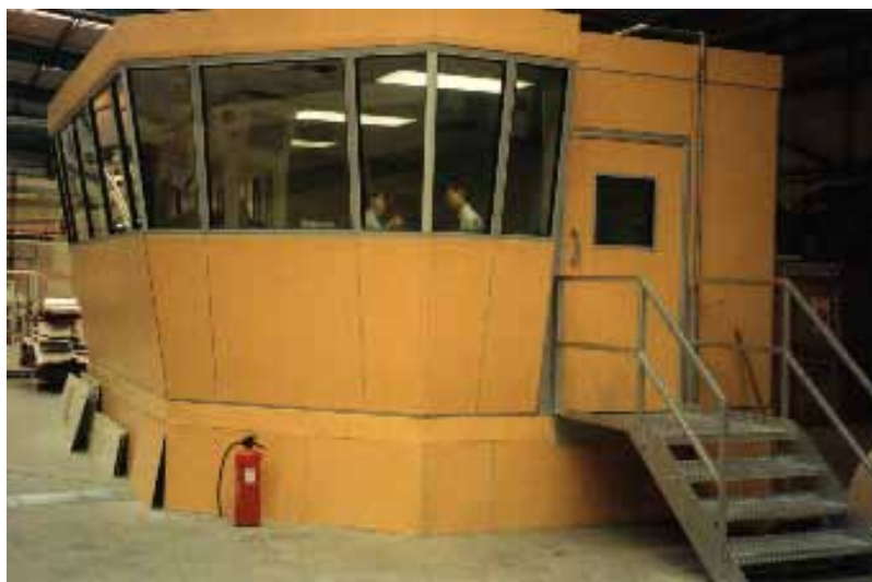
Figure 12 A noise refuge and control room
