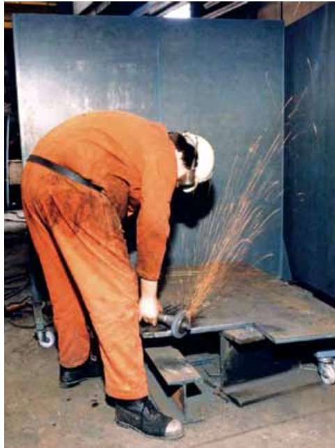
Figure 10 Moveable acoustic screen in an engineering workshop
