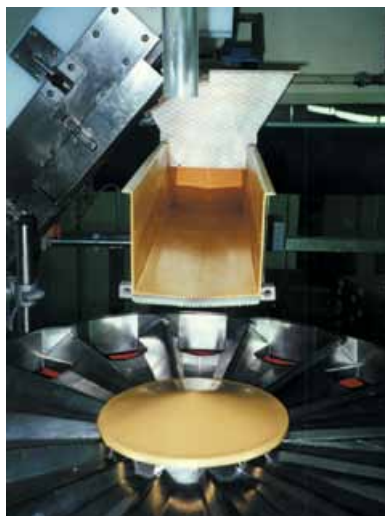
Figure 13 Damping material applied to transport chutes in the food industry
