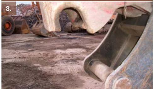
Safety pin is placed into position, this stops the jaws in no. 3 from accidentally being released
