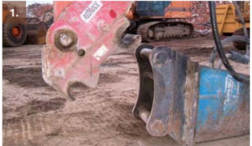
Quick release hitch being placed on the attachment
