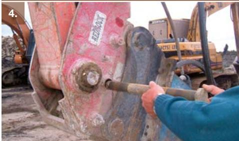
Safety pin in position with lynch pin to keep the safety pin in place
