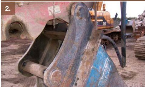
Ram pushes a set of jaws around the pin of the attachment
